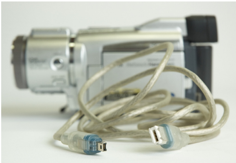
Figure 1-3: Plug the larger end of the FireWire cable—the six-pin end, as Apple calls it—into the corresponding jack on your Mac. The tiny end may look almost square, but it's not—it plugs into your camcorder only one particular way, thanks to a little indentation on one side. Be gentle with it.
