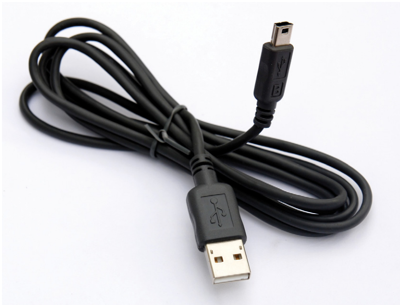
Figure 1-7: Tapeless camcorders generally come with a USB cable. The small end plugs into your camcorder (you may have to open some tiny plastic door on the camera to find the jack). The big end plugs into any of your Mac's USB jacks.
