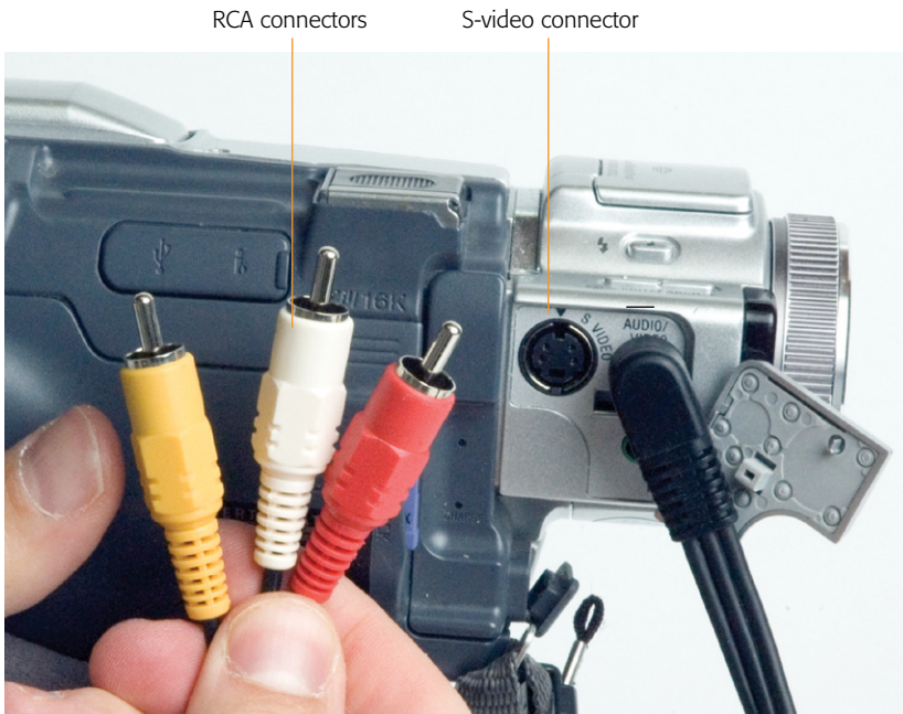
Figure I-2: Certain tape camcorders offer inputs for older, analog video. (Actually, what you'll probably get is a special cable with RCA connectors on one end and a miniplug on the camcorder end, like the one shown here. Don't lose this cable! You also need it to play your camcorder footage on TV.) A few older models offer an S-video connector too, for much higher-quality playback on TV.
